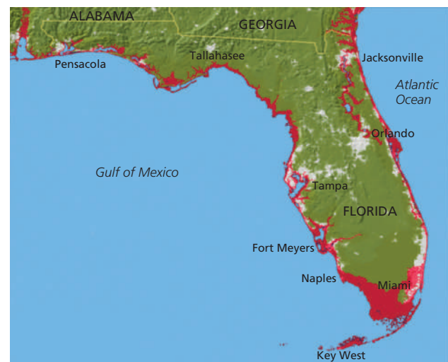
Figure 19-8 Areas of the U.S. state of Florida that will be flooded (red) if the average sea level rises by 1 meter (3.2 feet). (Data from Jonathan Overpeck and Jeremy Weiss based on U.S. Geological Service Data)
