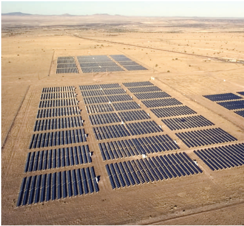
Figure 16-19 Solutions: This solar-cell power plant in the U.S. state of Arizona near the city of Springerville has been in operation since 2000 and is the world's largest solar-cell power plant. Analysis shows that the plant, which is attached to the area's electrical grid, paid back the energy needed to build it in less than 3 years.
