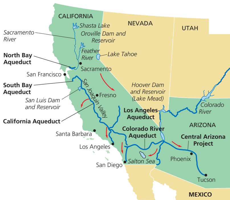
Figure 13-17 The California Water Project and the Central Arizona Project. These projects involve large-scale water transfers from one watershed to another. Arrows show the general direction of water flow.
