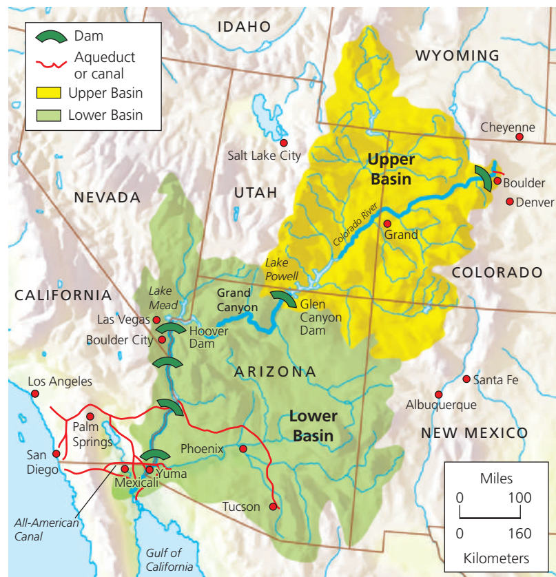
Figure 13-14 The Colorado River basin. The area drained by this basin is equal to more than one-twelfth of the land area of the lower 48 states. Two large reservoirs—Lake Mead behind the Hoover Dam and Lake Powell behind the Glen Canyon Dam—store about 80% of the water in this basin.
